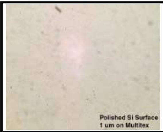
**Figure 9:** Image of the final polished Si surface following polishing on MultiTex polishing cloth. The surface appears relatively smooth with a few small scratches present. The dark spots on the image is contamination on the objective lenses.
